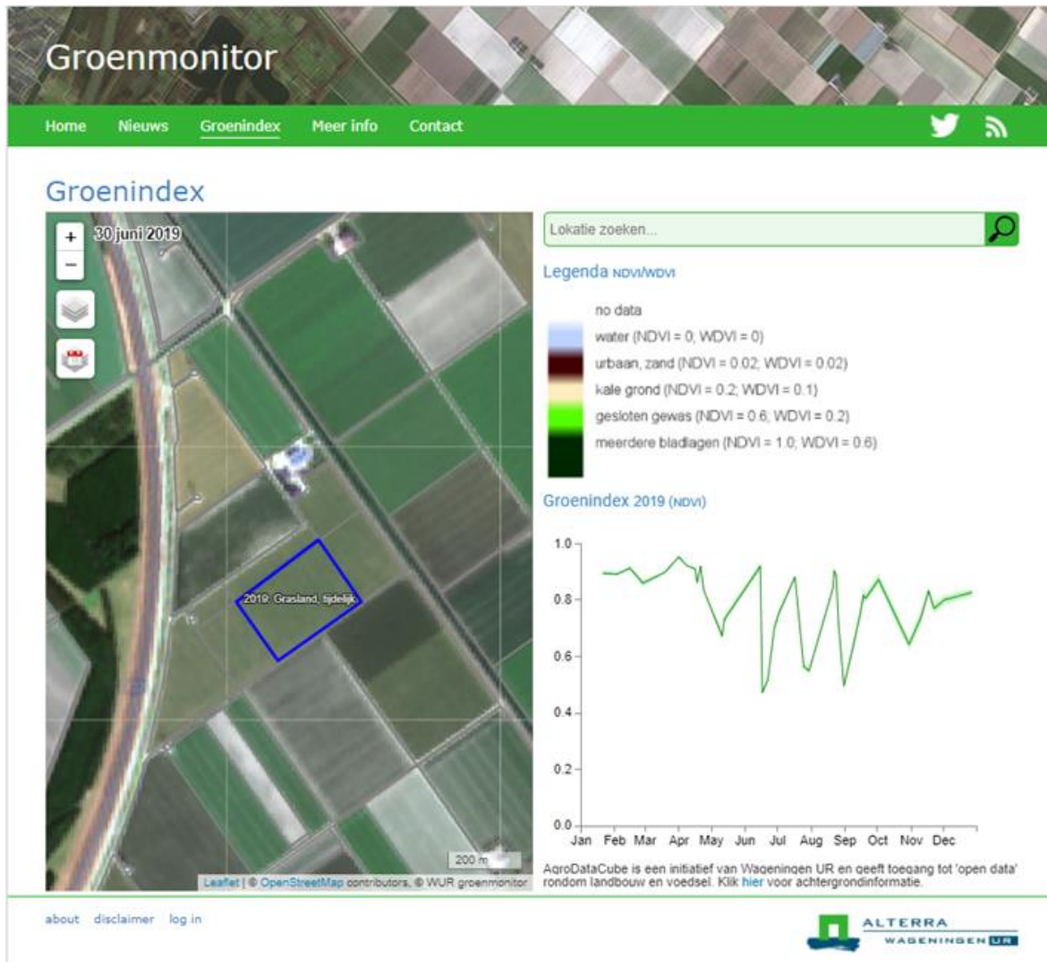
Figure 2: Screenshot of the Green Monitor ( www.groenmonitor.nl ). The graph shows the annual NDVI behaviour in 2019 of the blue marked grassland parcels (note that 5 mowing events can be distinguished).
